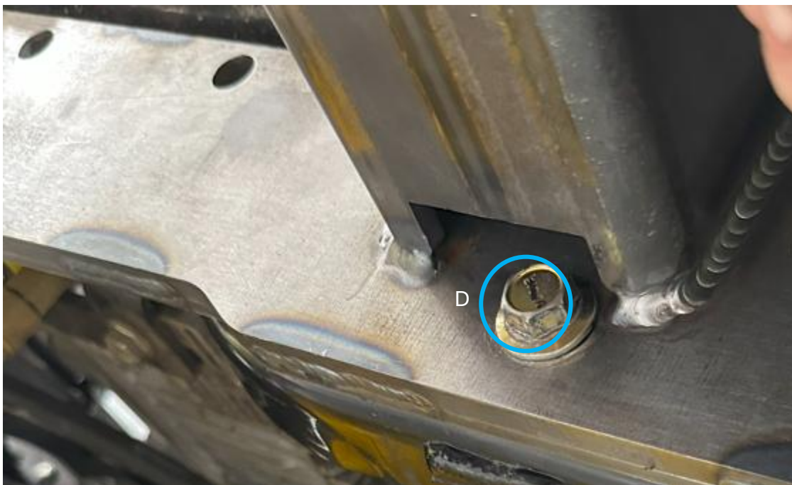
Figure 44: Installation of bolt in BLUE-D hole
