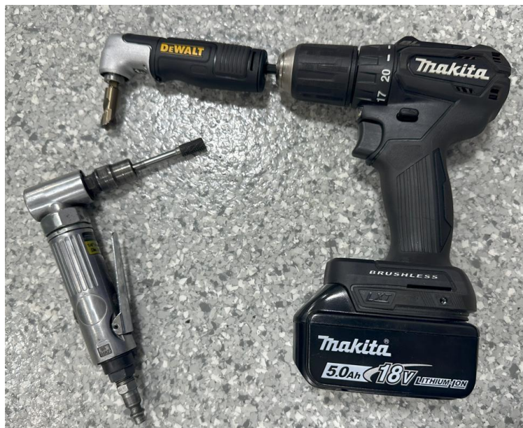
Figure 13: Tools that could be used to enlarge right side RED_J hole.
