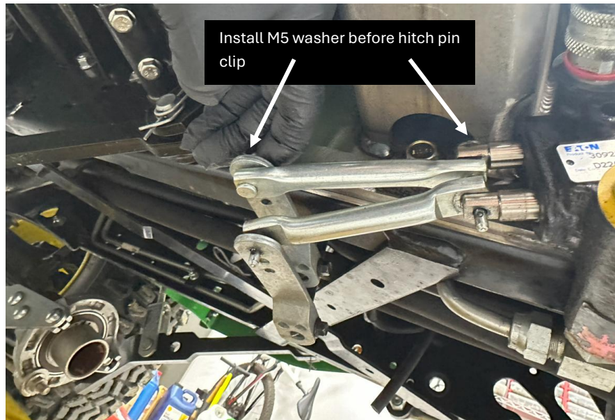
Figure 32 - SCV Linkage Installation
