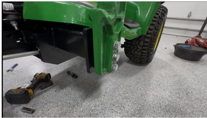
Figure 60: Installation of left side vertical mast
