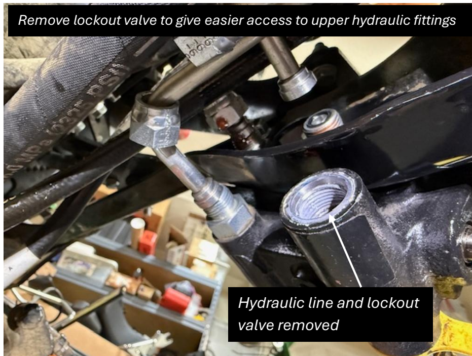
Figure 6: SCV Hydraulic line fittings
