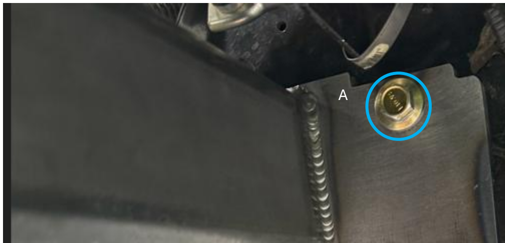
Figure 42: Supporting the rear of the mount with bolt in BLUE-A hole
