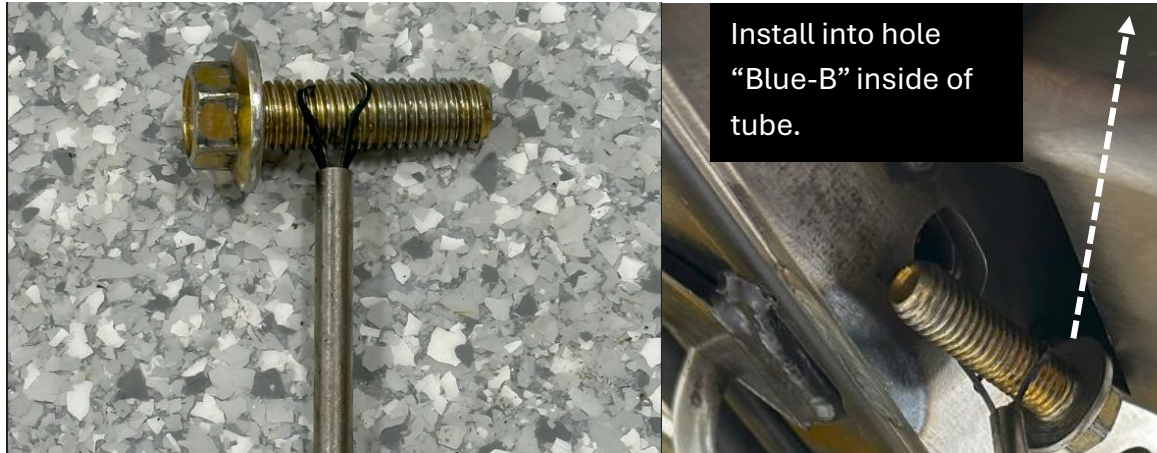
Figure 43: Tip to install blind bolt
