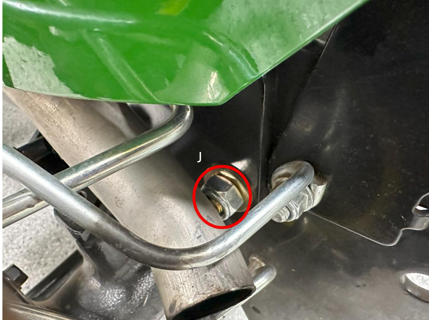
Figure 14: RED-J hole enlarged and bolt installed
