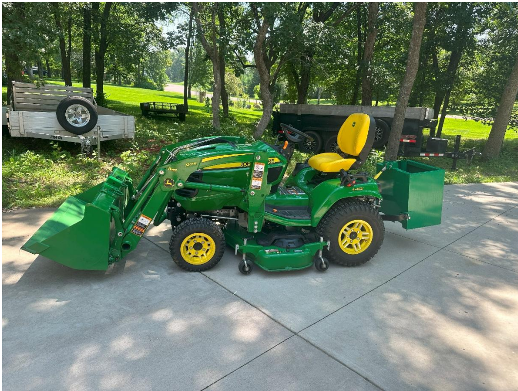
Figure 1: 2023 X739 with the 120R AWS Sub-Frame Mounts and John Deere 120R Loader
