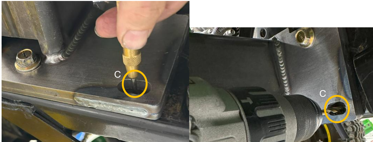
Figure 47: Marking and drilling of rear hole
