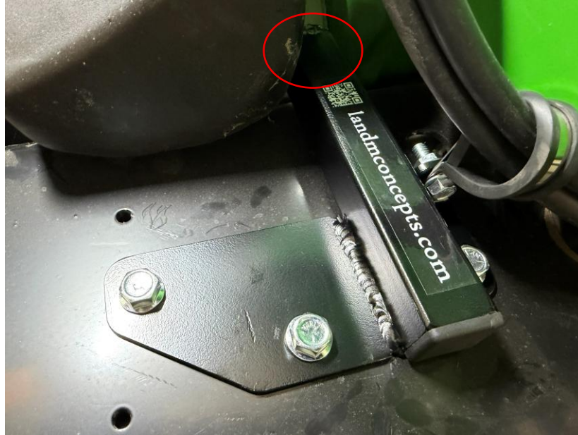
Figure 6 - Mast and cable clamp installed
