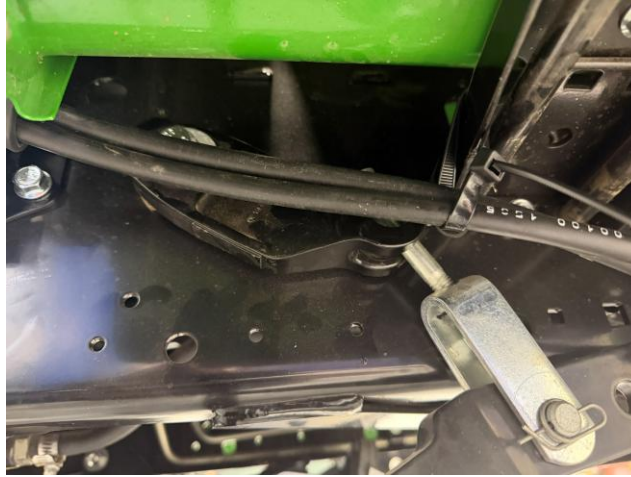
Figure 14: Retain cables from touching anything that moves.
