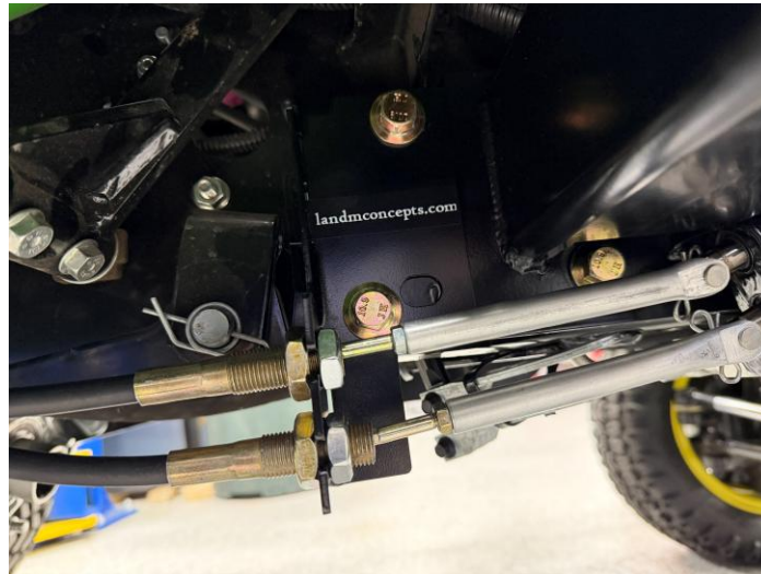
Figure 13: Connection of cables to retention bracket and SCV
