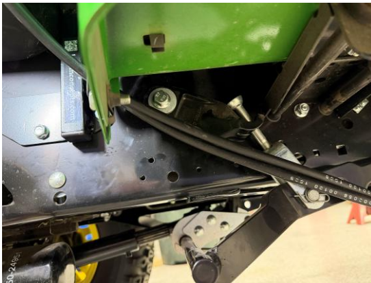
Figure 11: Route cables behind fender against frame.
