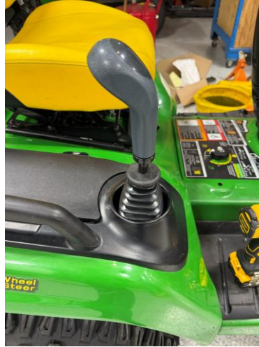
Figure 3: Initial orientation of Joystick handle upon installation.
