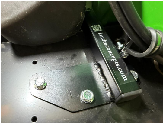
Figure 12: Retain cables near frame with cable clamp
