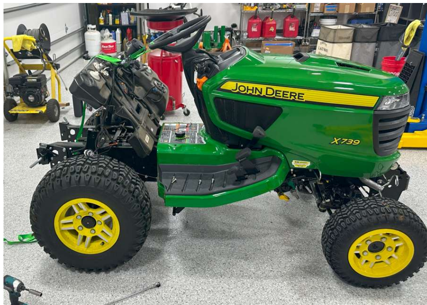
Figure 5: Fuel Tank tilted up and out of the way.
