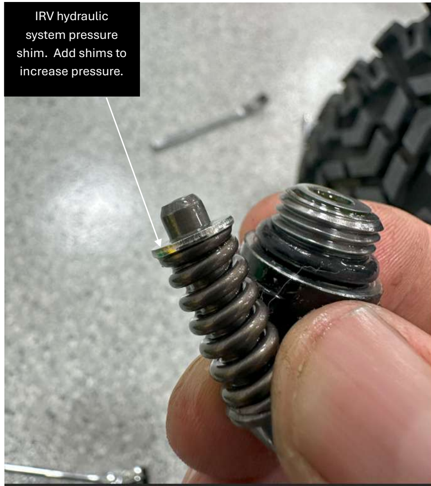
Figure 8: Implement Relief Valve (IRV) and factory shim
