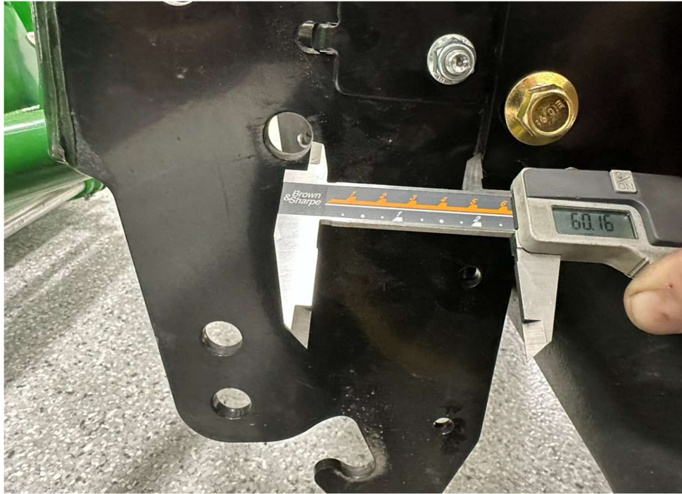
Figure 5: Alignment measurement front to back
