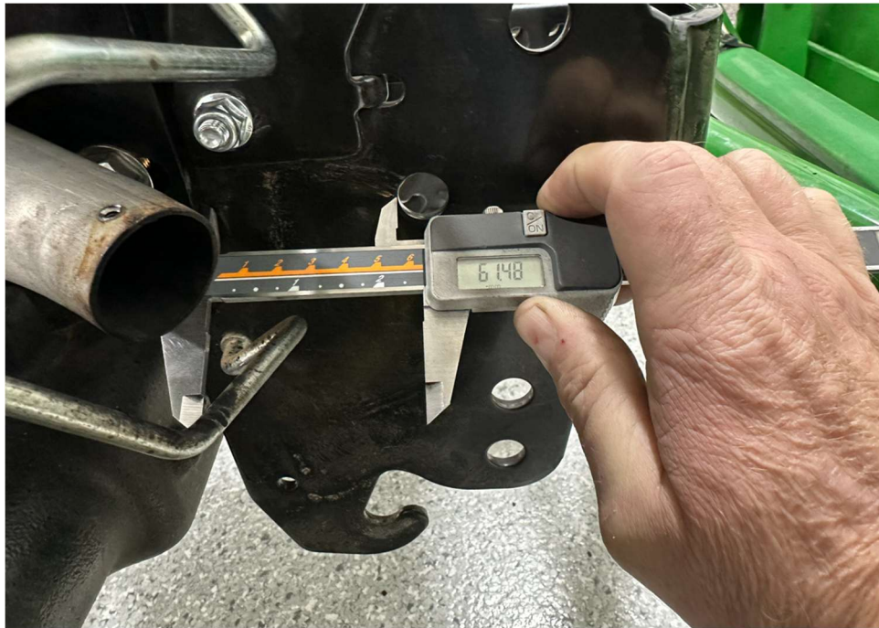
Figure 8: Right side mount alignment front to back.
