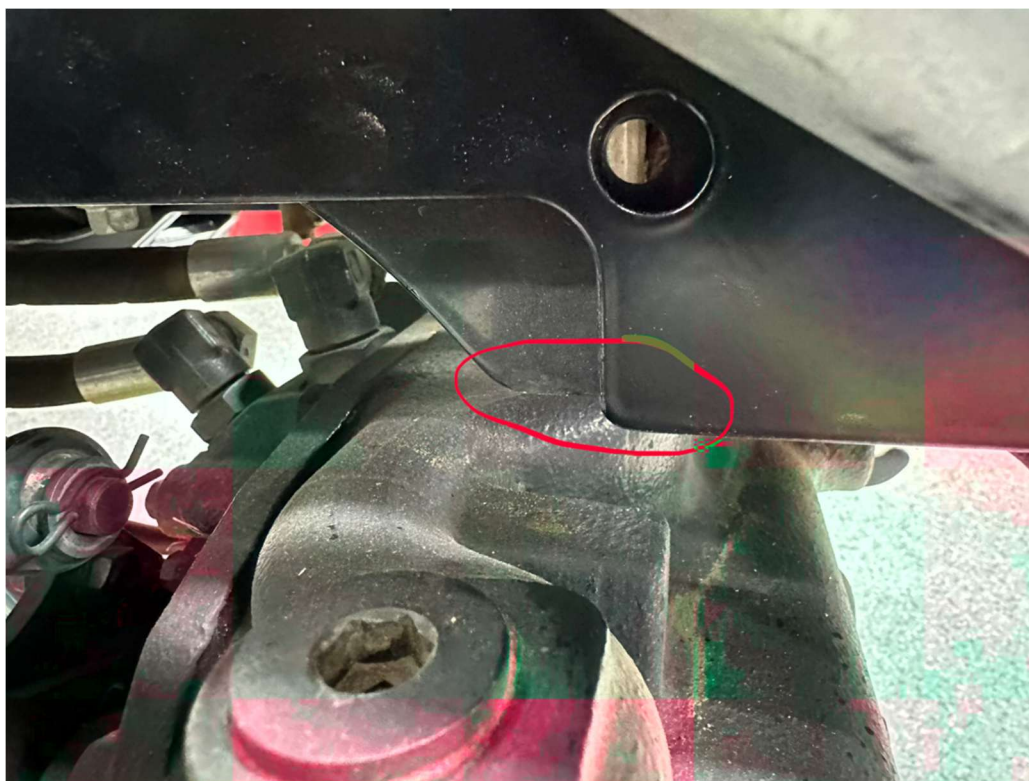
Figure 4: Bottom of Mount flush with Bottom of Frame (Right side shown - same for left side)
