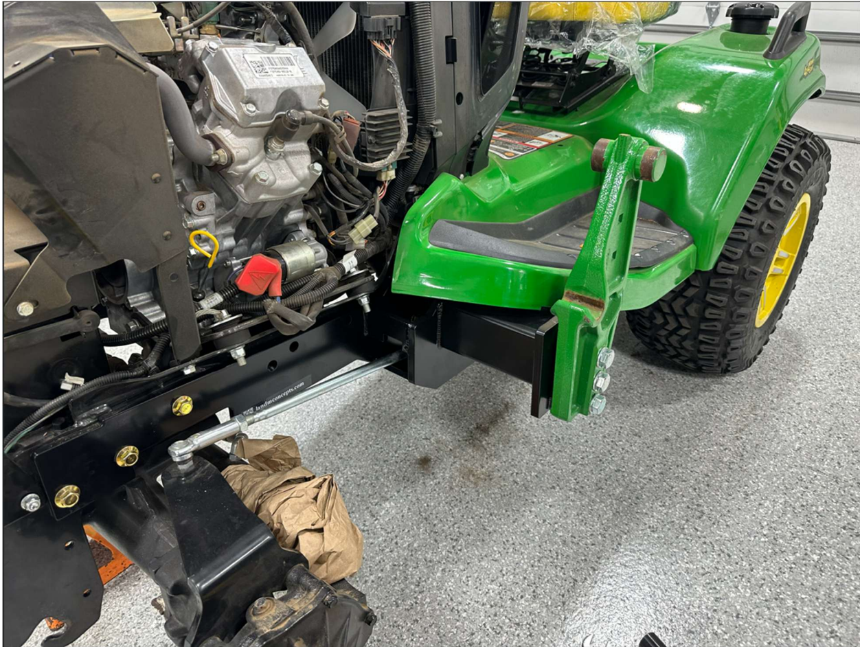
Figure 6: All bolts installed and torqued. AWS shown. 2WS the same.
