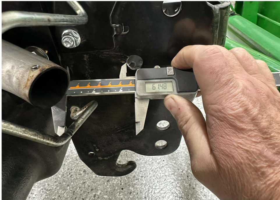
Figure 8: Right side mount alignment front to back.
